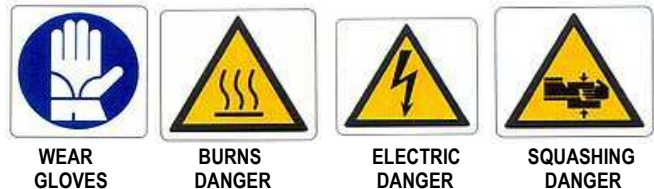
Label on machine's components showing potential dangers
